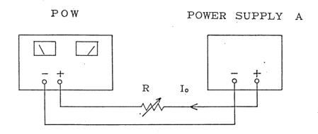
In such an operation, maximum current of POW is restricted to the value lower than generally using. Maximum allowable output current Io max is shown as follows.
