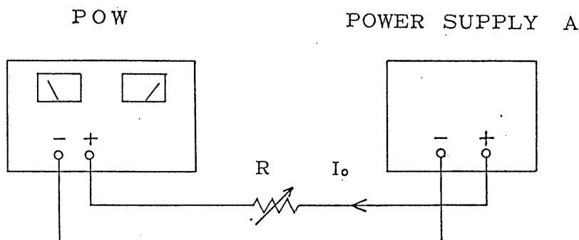
In such an operation, maximum current of POW is restricted to the value lower than generally using. Maximum allowable output current  $I_o$  max is shown as follows.
